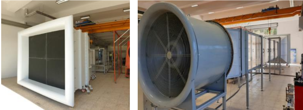
Figure 2.1. METU C3 open-return boundary layer wind tunnel facility at the center for Wind Energy Research (METUWIND).
